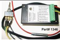
Turn signal relay system. This system is a great way to add turn signals to your classic car discretely. It is actuated by a small toggle switch. Turn signals will self-cancel after 15-180 seconds (adjustable). Capable of blinking both park and brake lights. Works on 12 or 6 volts, positive or negative ground.
